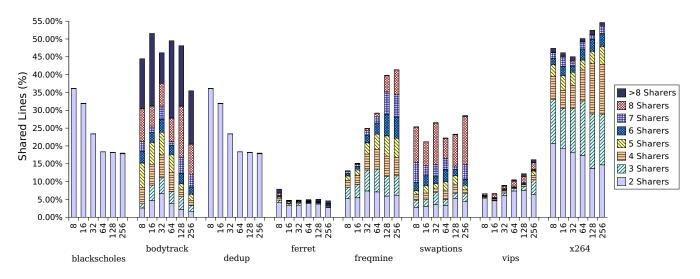
Figure 5: Portion of a 4-way associative cache with 4 MB capacity which is shared by 8 cores. The line size is varied from 8 to 256 bytes.
