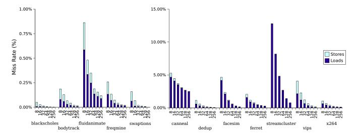
Figure 4: Miss rates as a function of line size. Data assumes 8 cores sharing a 4-way associative cache with 4 MB capacity. Miss rates are broken down to show the effect of loads and stores.
