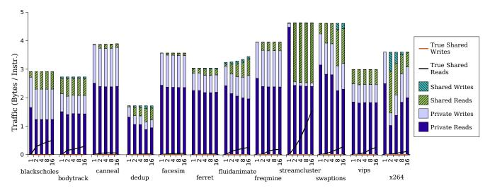
Figure 6: Traffic from cache in bytes per instruction for 1 to 16 cores. Data assumes a shared 4-way associative cache with 64 byte lines.
