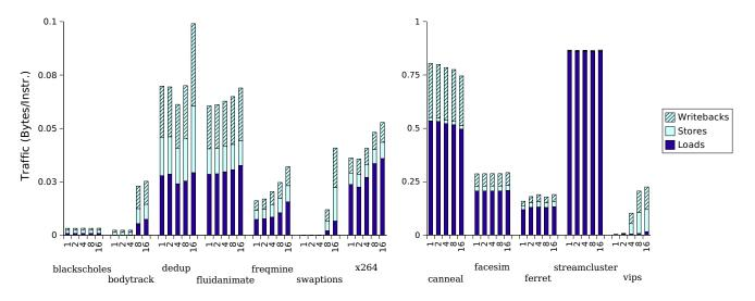
Figure 7: Breakdown of off-chip traffic for 1 to 16 cores. Data assumes a 4-way associative 4 MB cache with 64 byte lines, allocateon-store and write-back policy.
