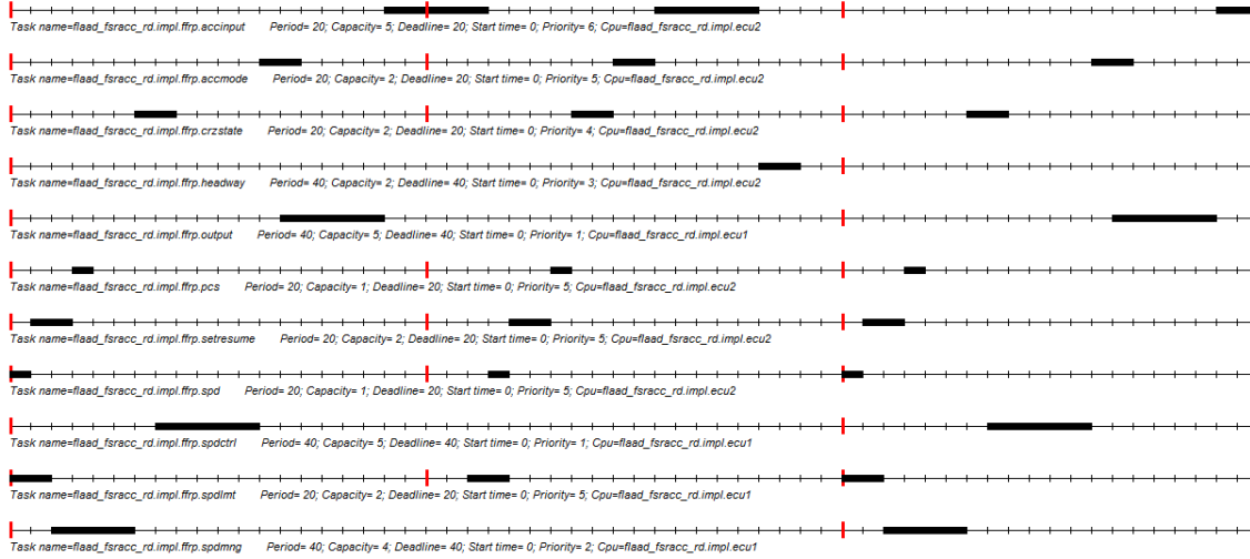
Figure 5. Cheddar simulation results of shared data access for dual-core setup.
