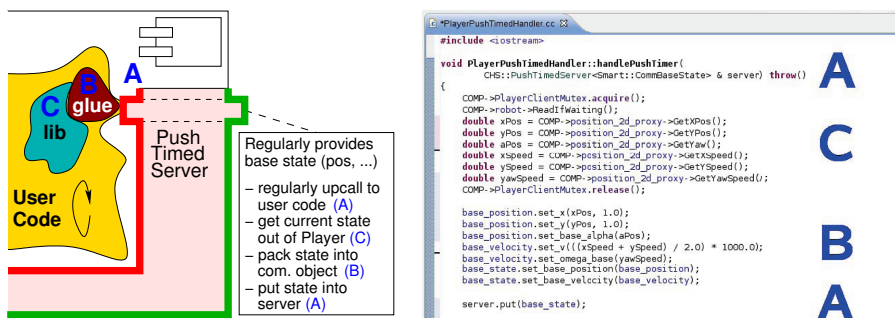
Fig. 4. Glueing user-code to service ports: example of a service port (based on a push-timed pattern) to regularly provide the base state (pose, velocity)
