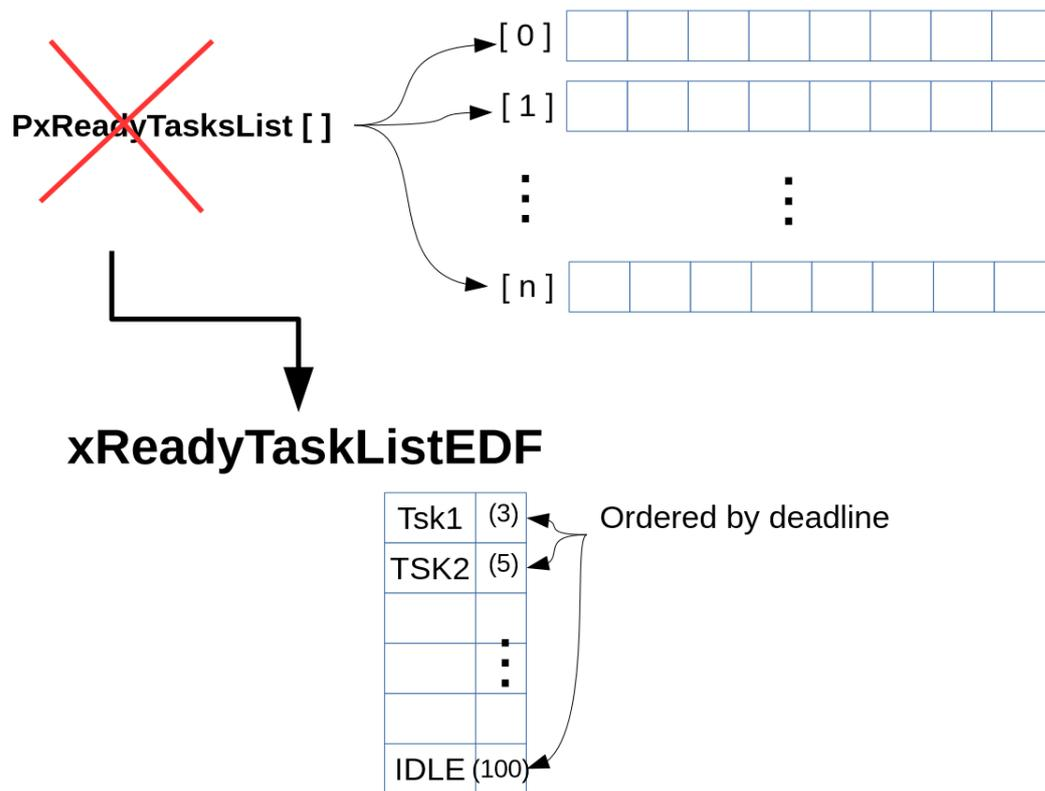
Figure 3.3: The new Ready List contains tasks ordered by increasing deadline time. The head of the list contains the task with the closest deadline
