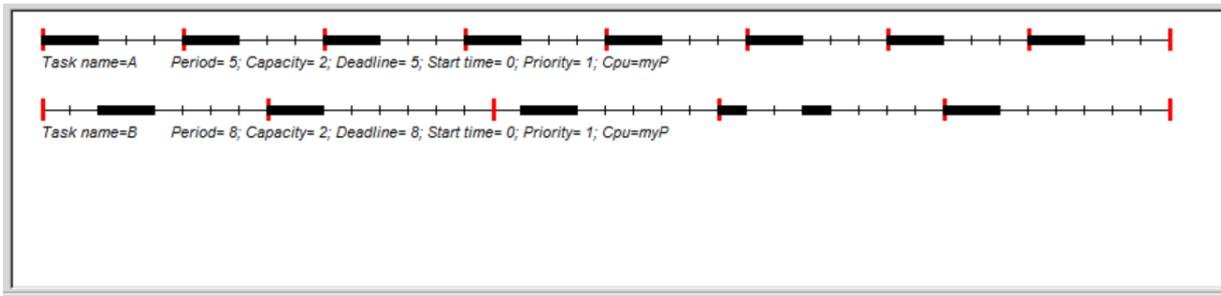
Figure 3.1: EDF scheduling of task A and task B
