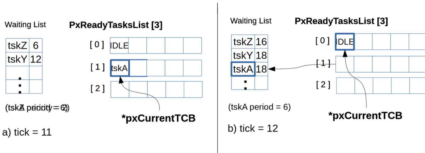
Figure 2.7: graphic representation of Ready List and Delayed List
