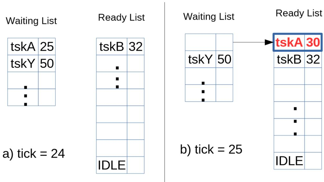
Figure 3.6: a) tskA will be awoken at the next tick. tskB has the nearest deadline among the tasks in ReadyList, so it's in the head position. IDLE is the task with the farrest deadline. b) After the tick interrupt happened, tskA moves to the Ready List:  $tskA_{deadline} = currentTick + tskA_{period} = 25 + 5 = 30$
