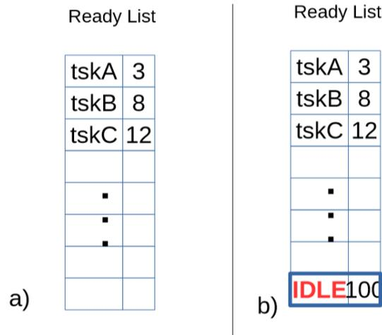
Figure 3.5: a) *tskA*, *tskB* and *tskC* are created before the scheduler is started; b) *vTaskStartScheduler()* method is called, the real time kernel tick processing starts and the IDLE task is added at the last position of the Ready List. It will execute only when no other tasks are in ready state.
