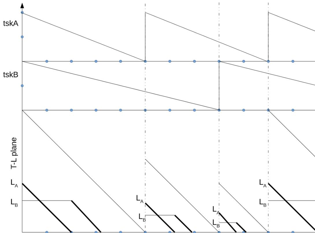
Figure 4.10: T-L plane construction for task A ( $p=5$ ,  $c=2$ ) and task B ( $p=8$ ,  $c=2$ ); For T-L plane 1:  $L_A = 2$ ,  $L_B = 1.2$ ; For T-L plane 2:  $L_A = 1.2$ ,  $L_B = 0.7$ ; For T-L plane 3:  $L_A = 0.8$ ,  $L_B = 0.5$ ; For T-L plane 4:  $L_A = 2$ ,  $L_B = 1.2$ ;
