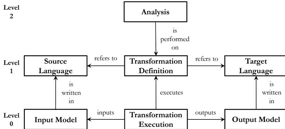
Fig. 2: Model transformation workflow implemented in Ocarina.
