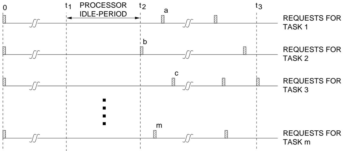
Figure 3: Processing overflow following a processor idle period
