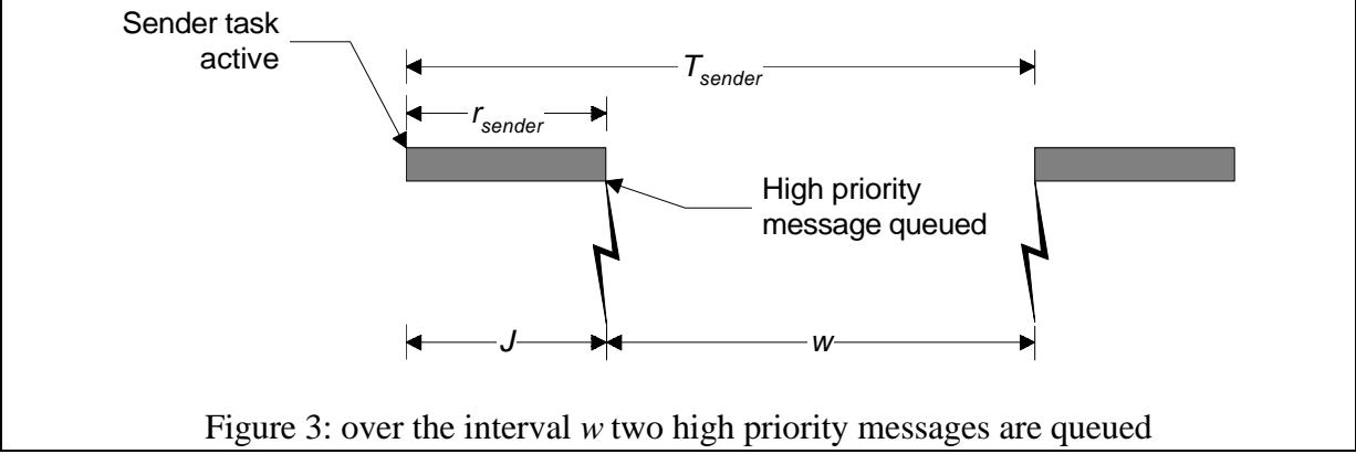
In Figure 3 the dotted boxes represent the worst-case release jitter of the sending task and the queued message; the high priority message has a release jitter of  $J_m$  (equal to the worst-case response time of the sender task) and a period of  $T$ .
