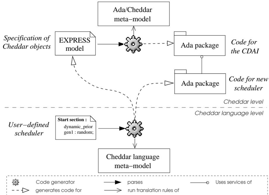
Fig. 5. Cheddar code generating from models and meta-models
