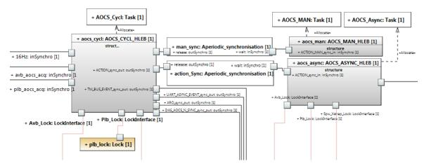
Figure 6 : Dynamic Architecture of AOCS\_Appli (UML Composite Diagram)
