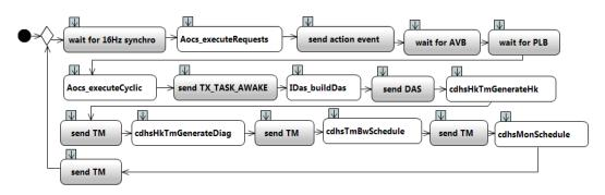
Figure 8 : Control Flow of AOCS\_CYCL High Level Execution Block
