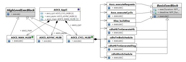
Figure 5 : Execution Blocks Definition (UML Class Diagram)
