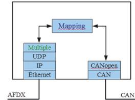
Figure 4. A (N:1) Gateway functioning
