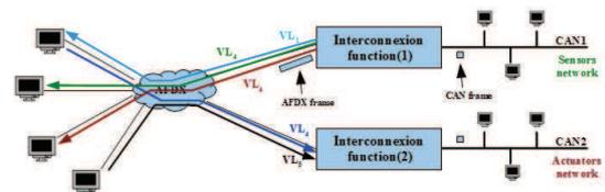
Figure 1. Interconnection of CAN buses to an AFDX backbone network
