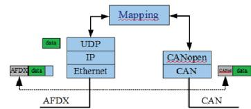
Figure 2. A (1:1) Gateway functioning
