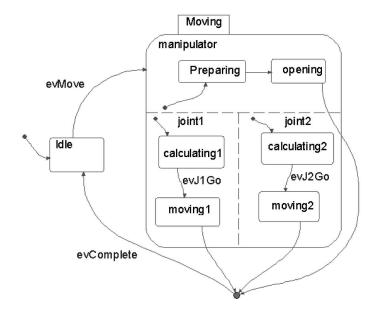
Figure 9: State diagram of a robot arm/manipulator
