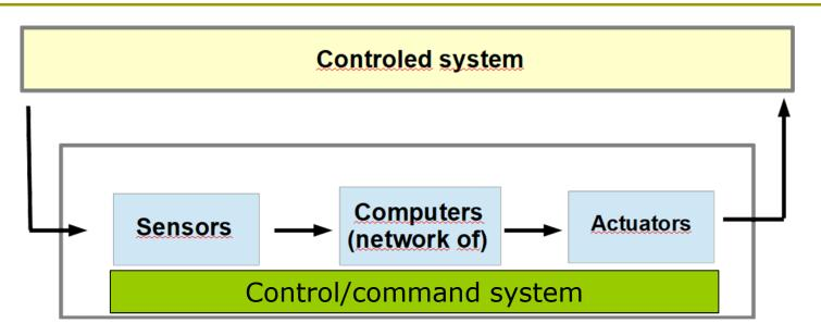
Real-time control and command software: computing system/programs which reacts in a given time 1) from sensor inputs 2) to send commands to actuators.
