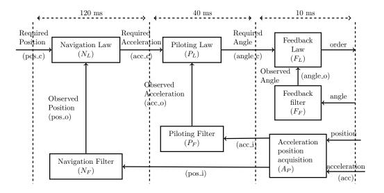
FIG. 1 – Flight control system
