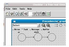
Make a simulation and verify that the precedences imposed by the messages are respected. To compute the response time, use the menu : Tools  $\rightarrow$  precedencies  $\rightarrow$  end-to-en response time  $\rightarrow$  compute and update tasks : one step. Apply this computing several times, until you find a fixed point. The underlying algorithm is the *holistic method* [TC94]. How do you interpret the results?
