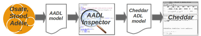
Fig. 2: Cheddar and analysis tool chain: AADL models are designed and are verified by AADL Inspector. They are translated to Cheddar-ADL to perform scheduling analysis with Cheddar.
